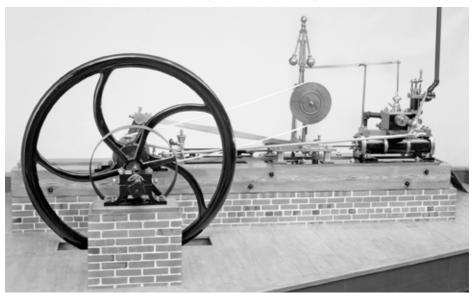
With a wooden bed, separate bases for the engine and the 79-inch flywheel, and refined decoration that extends to the Watt governor, the engine is considered indicative of the early days of American steam power. It was offered by Faber as an off-the-shelf stock item and spent the bulk of its working life in tanneries in Ohio and Kentucky.
