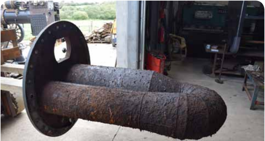
The firebox sees the light of day for the first time in twenty years. Note the complex shape as the firebox cylinder narrows to join the lobster back bend and then narrows again to exit with the chimney dimension. The original would have been made from riveted small wrought iron plates.
