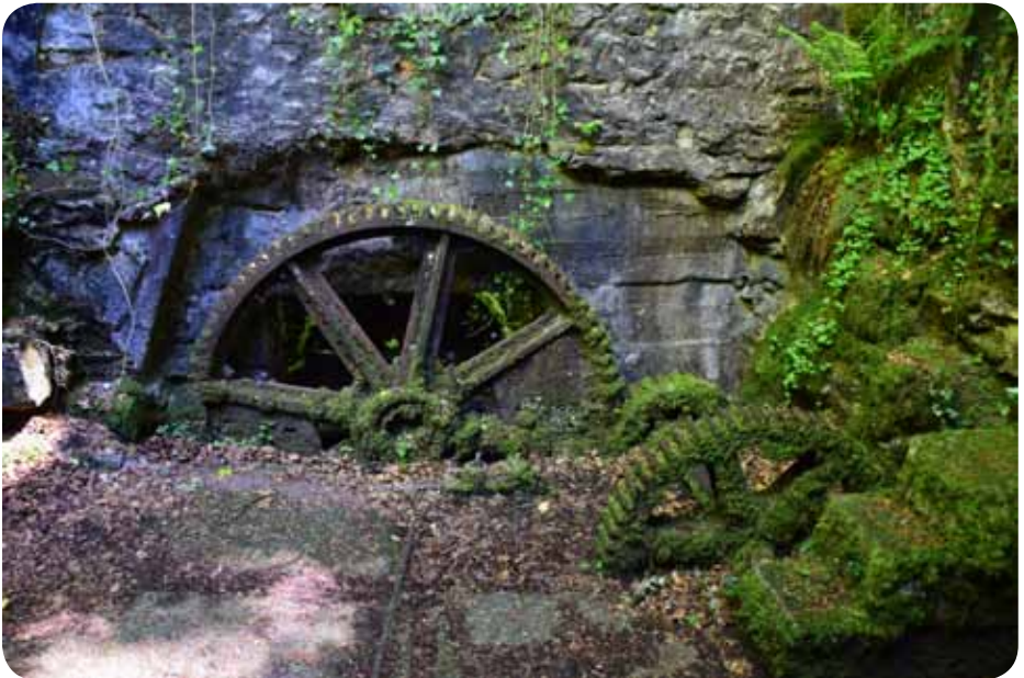
The remains of the overshoot waterwheel which sat between two mills massively constructed of granite blocks. The remnant gearing seen below was in a room below the mill bed, to reduce the risk of explosion. The roof of these mills was flimsy so any such explosion was directed to the heavens.
