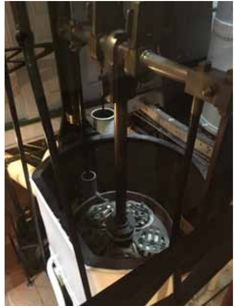
Figure 12: Ticonderoga's hotwell, air pump, air pump rod, crosshead, crosshead guides and linkage to the connecting rod by which it was operated.
