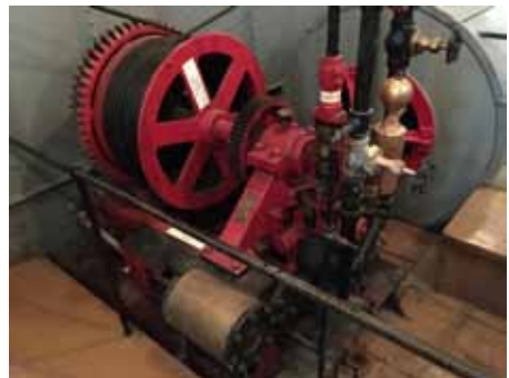
Figure 14: Ticonderoga's auxiliary blower engine (left) and power steering engine (right).
