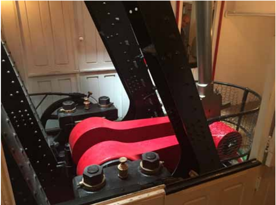
Figure 10: View of Ticonderoga’s paddlewheel crank and connecting rod.
