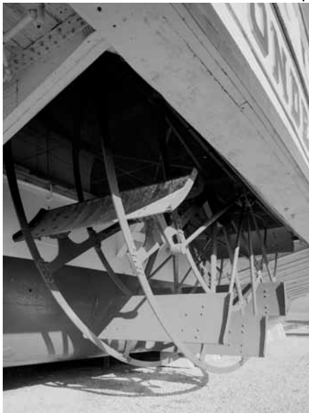
Figure 3: Views of the Ticonderoga's port (right) and starboard (left) Morgan feathering paddlewheels, the 1988 HAER photograph (right) showing five of the ten buckets (U.S. Library of Congress).
