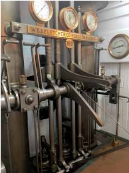
Figure 11: Ticonderoga's in-line, two-piece arbor, eccentric-arm operated valve gear (steam side pipe and steam inlet valves left, exhaust side pipe and exhaust valves right) with steam gauge (left), clock (centre), vacuum gauge (right) and crank indicator (far right); the latter used to prevent the engine from stopping on dead centre. Threaded lifters (centre) allowed the lower (left) and upper (right) steam valves to be adjusted. Paired handles to the left controlled the condenser water valves, whereas those to the far right controlled the boiler feed. The crank indicator was used to prevent the engine from stopping on dead centre. Inclined lever (lower right) is the starting bar.
