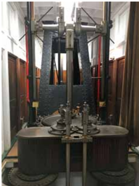
Figure 7: The Ticonderoga's top steam chest and valve nozzles, 53-inch cylinder top, piston rod, crosshead and crosshead guides.
