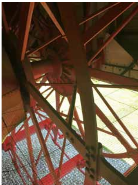
Figure 3: Views of the Ticonderoga's port (right) and starboard (left) Morgan feathering paddlewheels, the 1988 HAER photograph (right) showing five of the ten buckets (U.S. Library of Congress).
