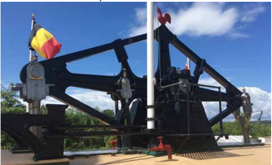
Figure 9: Diamond-shaped hollow-work beam on Ticonderoga's hurricane deck, showing linkages to the piston rod (left), hotwell and air pump (centre) and connecting rod (right). The rooster is not original but was added by Electra Webb for good luck.
